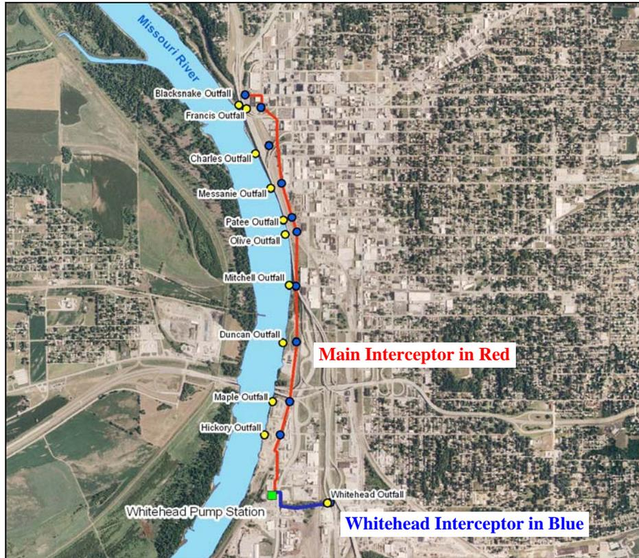
**Figure 1 – Plan View of Main Interceptor and Whitehead Interceptor**
