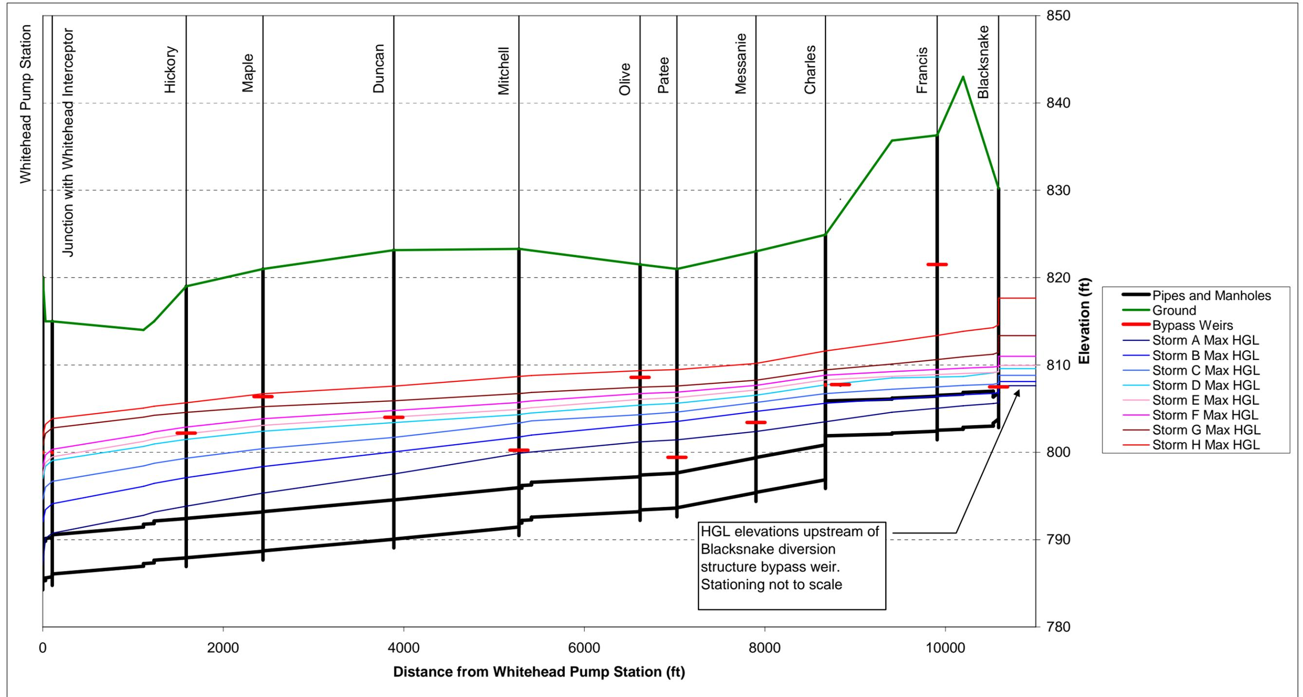
Figure 2 – Main Interceptor Profile for Typical Year Design Events after Phase IA Improvements
