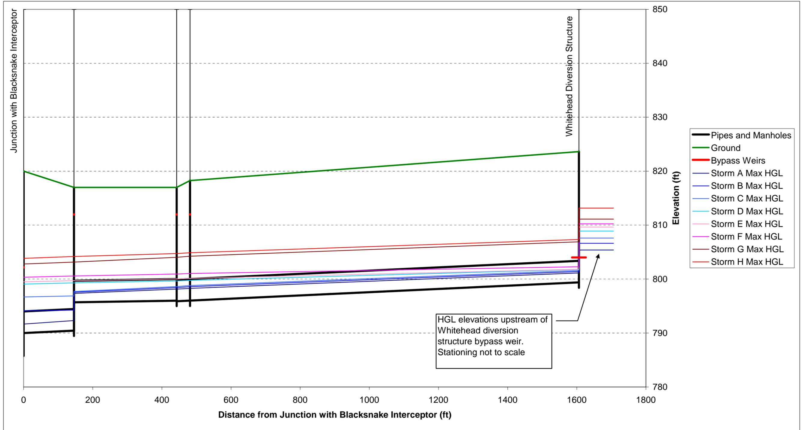
Figure 3 – Whitehead Interceptor Profile for Typical Year Design Events after Phase IA Improvements
